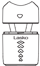
1. Turn counter clockwise to unscrew Top Cover
